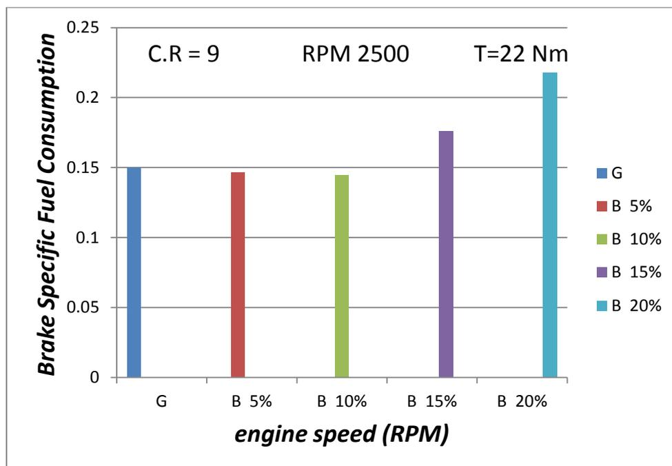
Fig.2 . Brake specific fuel consumption versus engine speed.
