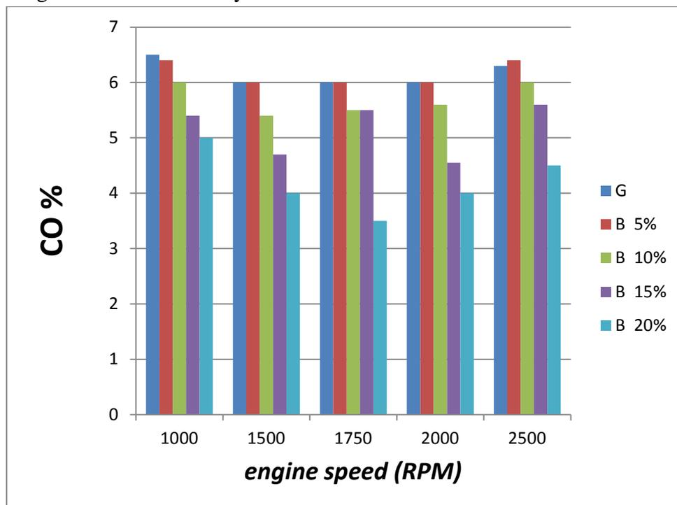
Fig. 4. Carbon monoxide versus engine speed.
