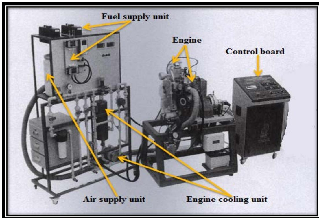
Fig (1): A photographic picture of the experimental rig
