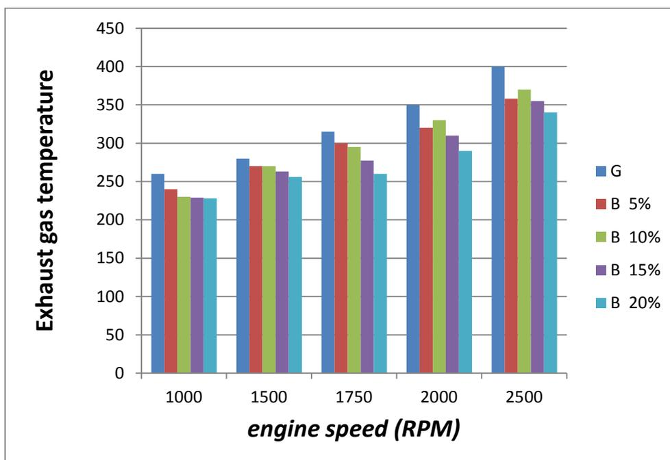
Fig. 6. Exhaust gas temperature versus engine speed.
