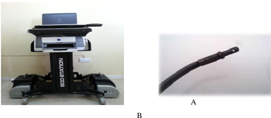
Figure (2): **A**— the exhaust gas analyser type (TEXA).
