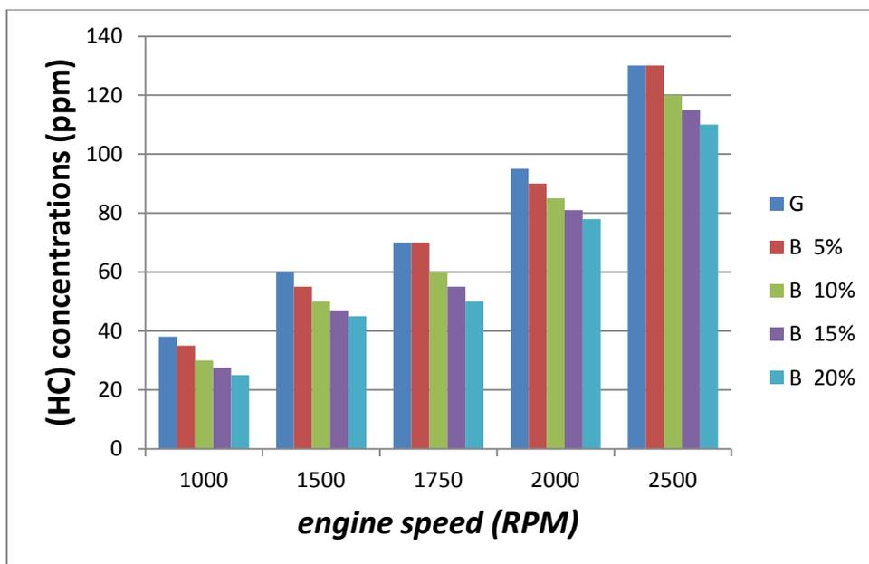
Fig. 5. Unburned hydrocarbon (UHC) versus engine speed.
