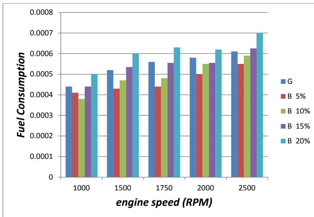
Fig 3. Fuel consumption versus engine speed.
