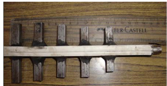
Figure 2(b) - Yagi-Uda Antenna using square iron rod as Antenna element.
