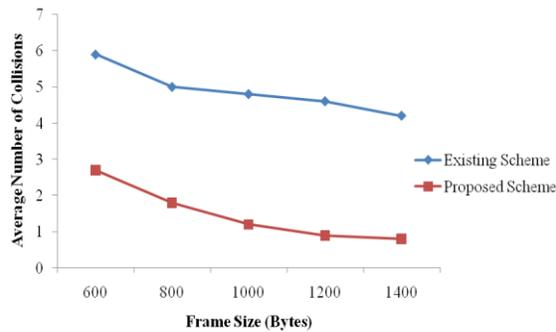
Fig. 6: Average Number of Collisions vs. Frame Size at 11 Mbps
