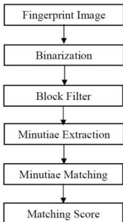
Fig: Fingerprint recognition steps
