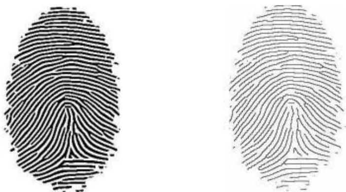
Fig. 5: Binarized and thinned fingerprint.
