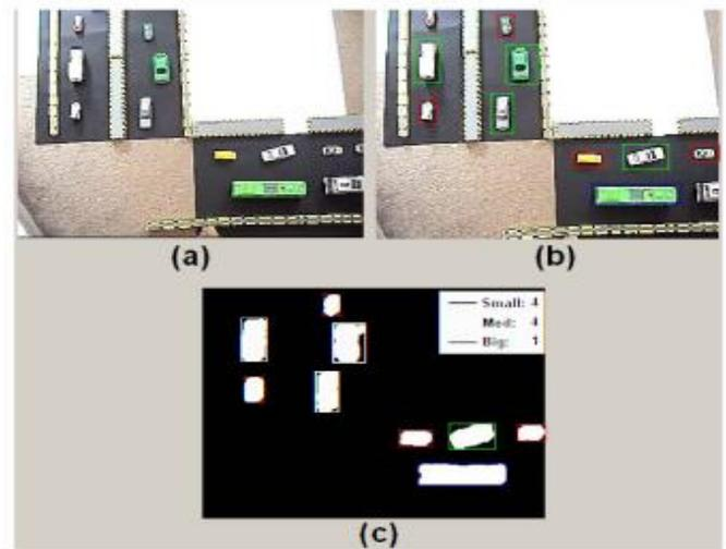
Figure 5. Detection and classification result (a) Original image (b) Detected vehicles (c) Image generated through the algorithm for vehicle detection and classification
