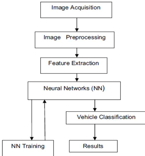
**Figure 13. Vehicle detection and classification scheme**
