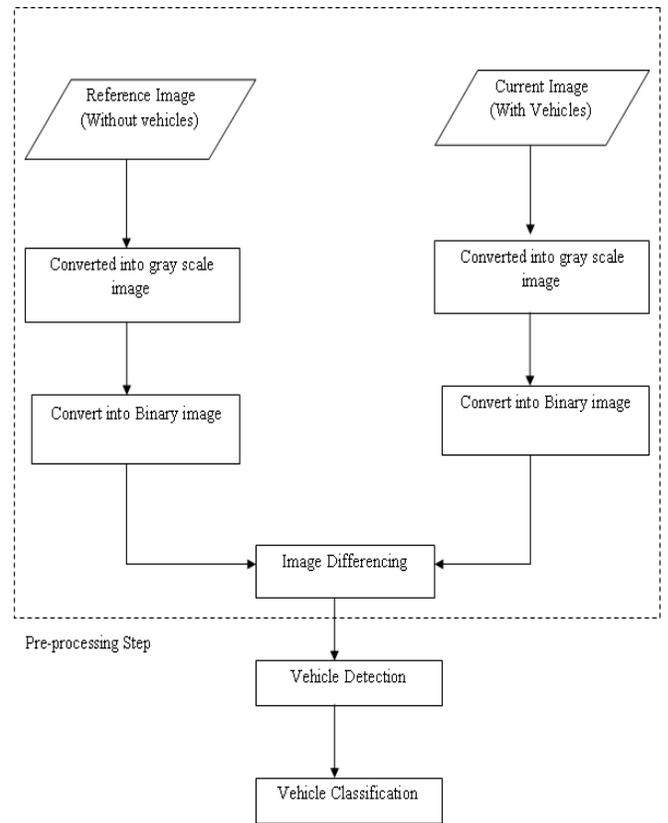
Figure 8. Flow diagram of a proposed System.
