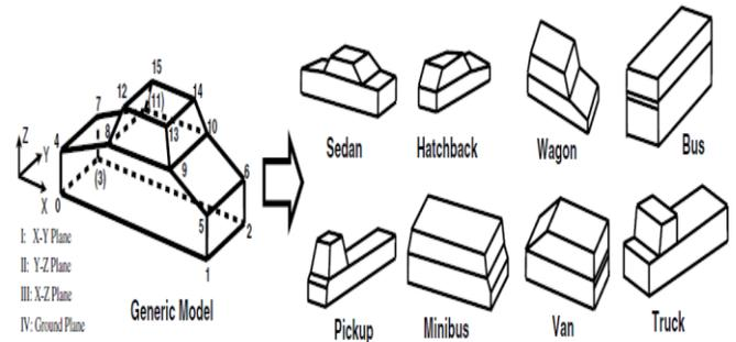
**Figure 2. A generic 3D vehicle models which can be deformed to fit with different vehicles**
