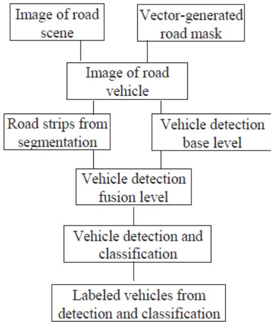
Figure 6. Flowchart based on object-oriented image analysis method.
