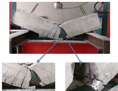
Figure 4: The Beam B0 after Failure
