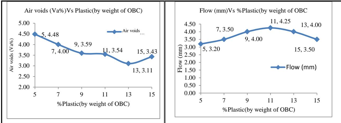
**Figure-6** - % Plastic Vs. Stability , Density, Air voids& Flow values values
