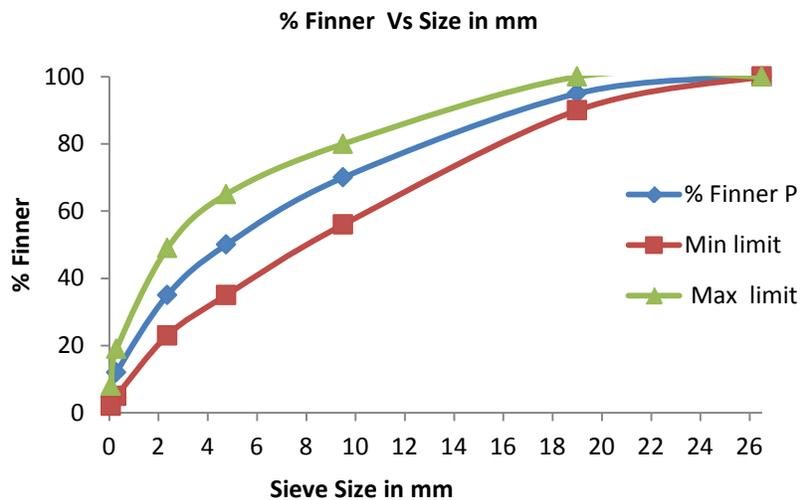
Figure-1 Gradation Curve for the aggregates
