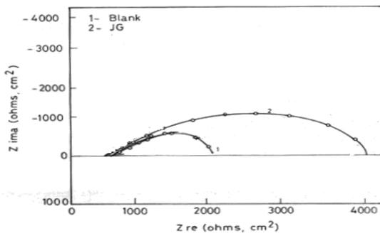
Figure 7: AC impedance diagram for mild steel in 0.005 M NaCl in the presence of 4% VCI
