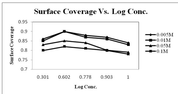
Figure 11: Temkin adsorption isotherm for 4% VCI based on VIA Test in NaCl environments for mild steel
