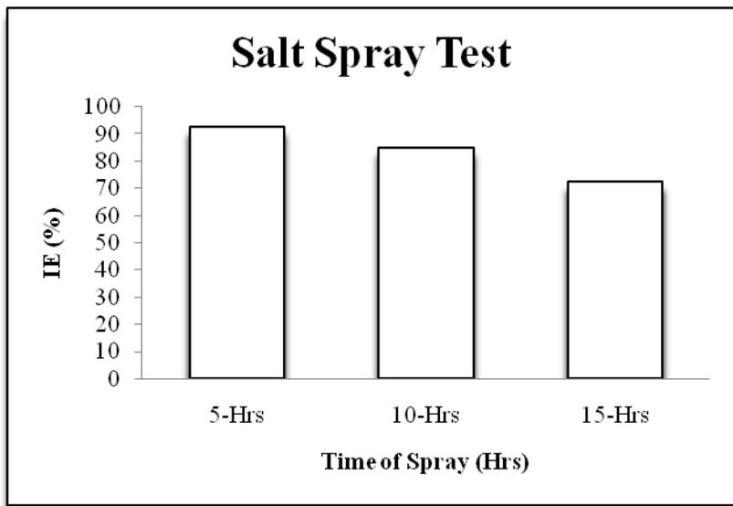
Figure 3: Inhibition efficiency for 4% concentration of VCI 3.5% NaCl environment under Salt spray test
