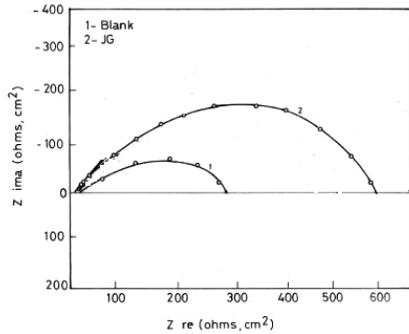
Figure 8: AC impedance diagram for mild steel in 0.05 M NaCl in the presence of 4% VCI
