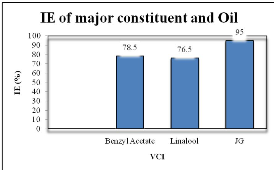
Figure 4: Inhibition efficiency for 4% concentration of major constituents based on VIA Test in 0.005 M NaCl environment
