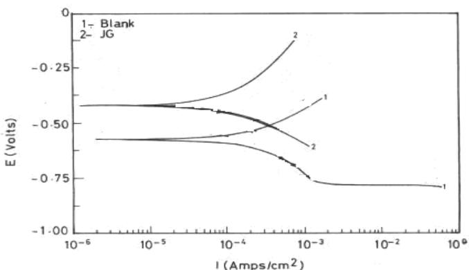
Figure 6: Potentiostatic polarization curves for the corrosion of mild steel in the presence of 4% VCI in 0.1M NaCl
