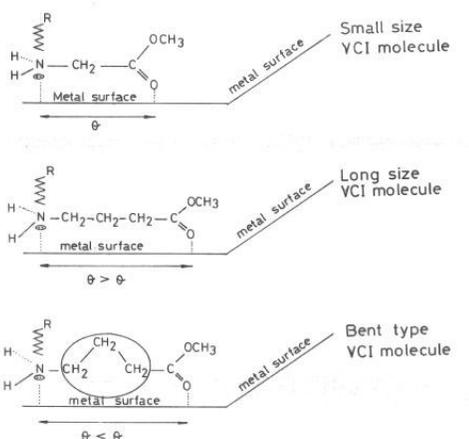
Figure 12: Schematic representation of adsorption of VCI on metal surface
