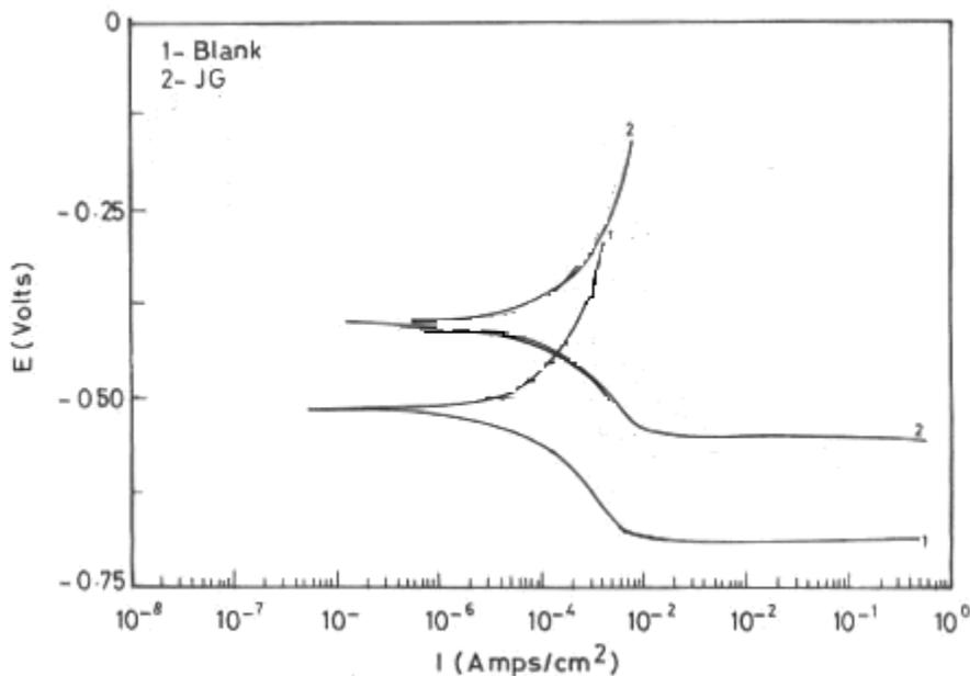
in 0.005 M NaCl environment. The corrosion current density ( $I_{corr}$ ) for the blank is 166.7  $\mu A/cm^2$ . The addition of inhibitor vapour results in a decrease in corrosion current density. The decrease in corrosion current density indicates that the cathodic protection takes
